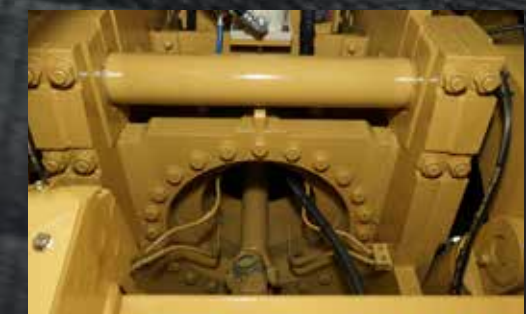
Heavy duty split mainframe with oscillating bearing frees axle pivot
