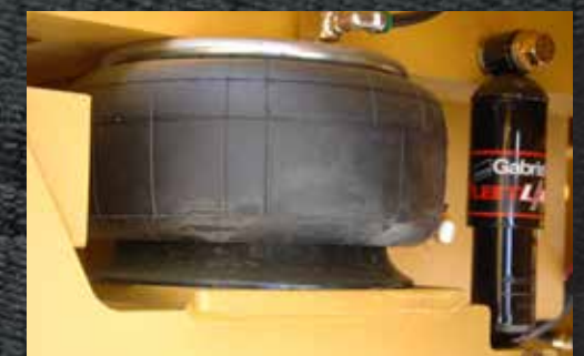
Goodyear® air springs, stabilizing shock absorbers, and isolation mounts
